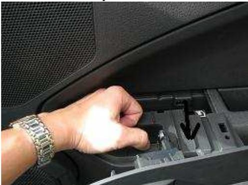
6. Remove the door lock bezel by slightly lift it up – a small screwdriver may be needed.
