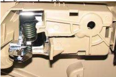
12. Remove the stock door handle from the cup by opening it to the full open position and prying up and down to pop it off the plastic studs in the handle cup.
