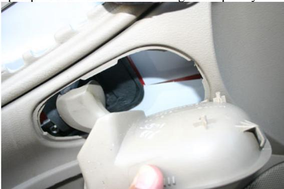
6. Using the side cutters or an appropriate saw or dremel type tool, cut the bottom of the roll pin used to hold the handle to the brace. Metal pieces may be ejected here at high velocity, so be careful and use appropriate safety precautions.
