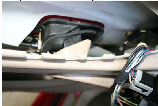
5. Using the hook tool or a flat screwdriver, pop the plastic cup from around the door handle – putting the handle in the open position will aid in removing it completely.
