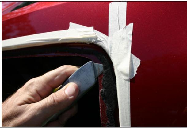
5. Clean and lightly scuff the application surface of the louver, and follow sealer's directions for proper preparation of louver surface with the correct adhesion promoter – this is very important to aid in achieving a satisfactory bond. When using 3M Fast Weld Urethane, the proper adhesion promoter is 3M Single step, P/N 08682, available separately – this can also be used to touch-up scratches on the pinch-weld if required.
